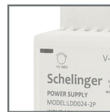
LED diode indicating the operation of the power supply
