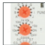
TR-U1P rotary switch to set functions and time ranges
